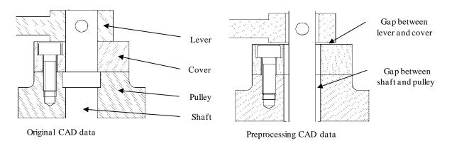
Figure 3. Changes in the CAD data (preprocessing)
