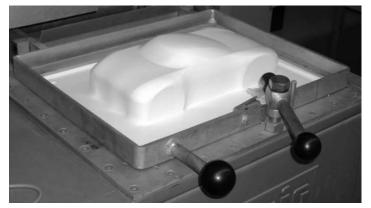
b. Thermoformed plastic sheet *Figure 7. Use of rapid tooling*
