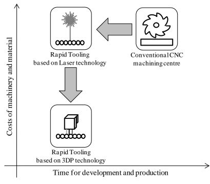
Figure 5. Comparison of different tool building methods
