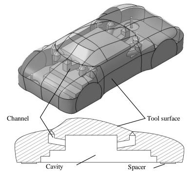
Figure 6. CAD model of a forming tool: 3D view and cross-section
