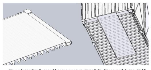
Figure 4. Loading floor and trapeze cross member (left), Goose neck tunnel (right)
