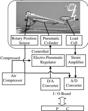
Figure 4. Control system of rehabilitation support device
