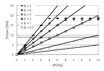
Figure 6. Experimental results of compliance control
