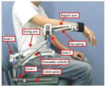
Figure 1. Independent support device
