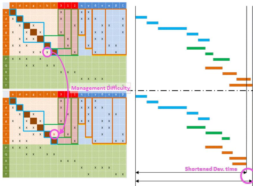
Figure 13. Comparison of process candidates with tradeoff between span and manageability
