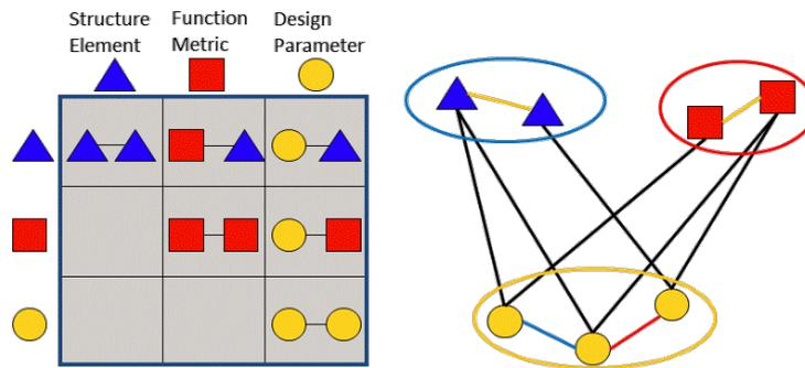
Figure 3. Relations among structure elements, function metrics, and design parameters in both matrix and network representations
