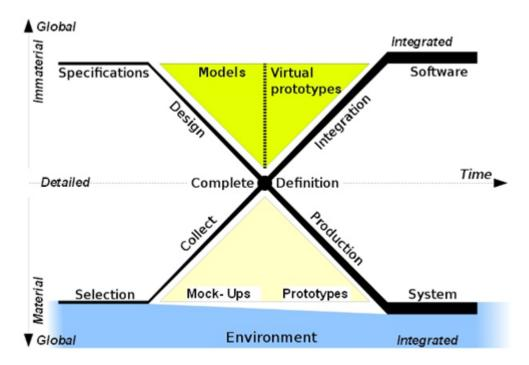
Figure 3 Scheme of the X-development method.
