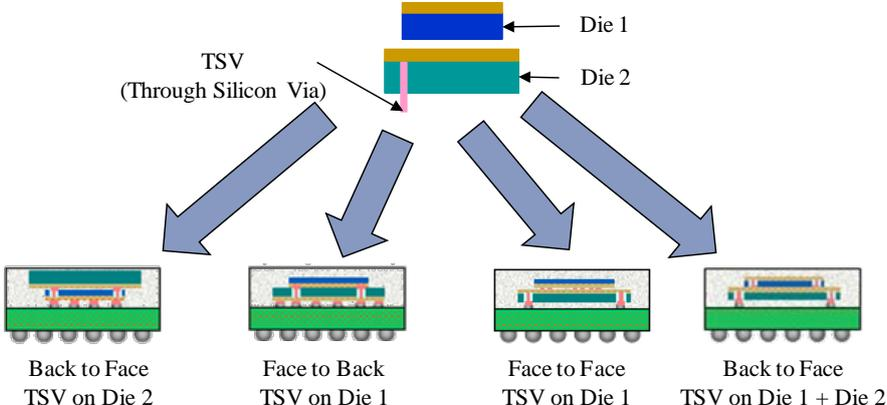
Figure 3: Device architectures as a C-K model output
