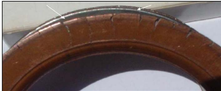
Figure 2. Metal bearings failure in manufacturing. Detachment areas shown by arrows.
