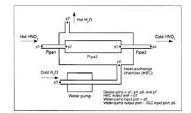
Figure 1. The structure of a nitric acid cooler [2]
