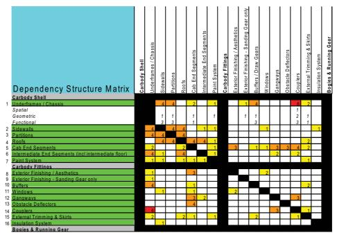
Figure 1. A section of the product interface connectivity model for a rail vehicle
