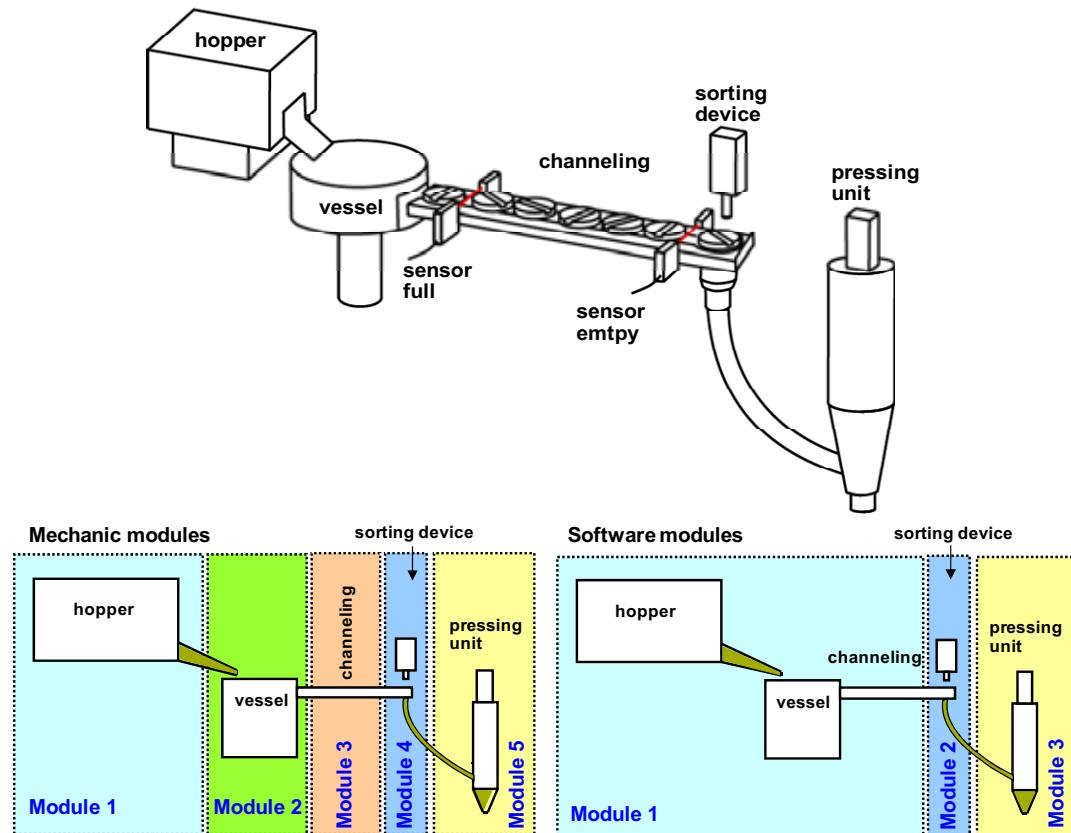
Figure 1. Exemplary modularization of the same machine in two different disciplines
