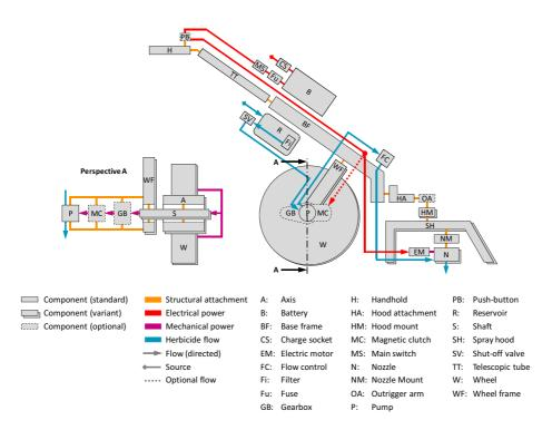
Figure 2. Visualisation of a spraying system by the Module Interface Graph (MIG)
