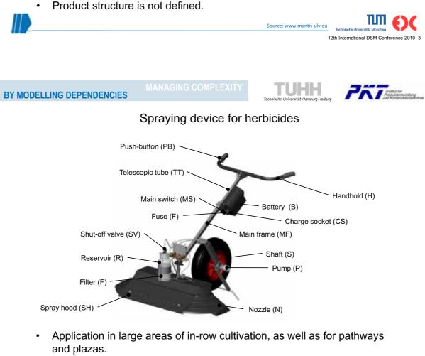
Ultra Low Volume (ULV-) technology allows the use of undiluted fluid.
