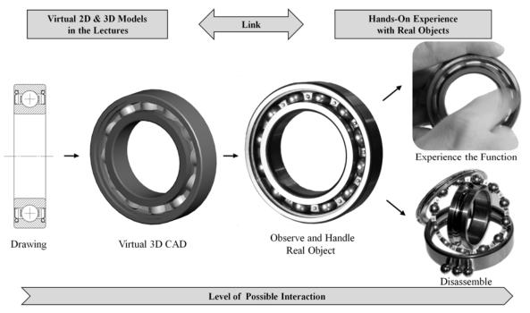
Figure 4. Abstraction from Real Object to a Technical Drawing
