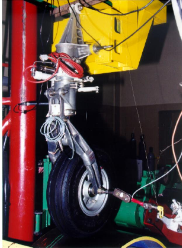
**Figure 4. A gear landing during the test**
