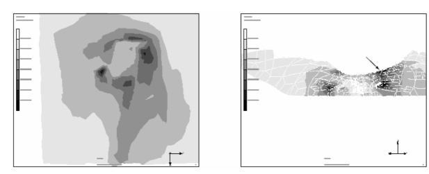
Figure 8. The left figure shows a typical pressure distribution pattern. for  $C_{10} = 500$  Pa and maximum load. The right figure shows a typical stress ( $S_{33}$ ) pattern in a vertical cutting plane along the length of the ischium
