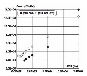
Figure 7. The relationship between the maximum pressure, the maximum displacement of the support, and the elasticity. The black squares show the results of the two-coefficient analysis; the circles give the displacement and the maximum pressure of the three-coefficient analysis
