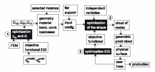
Figure 2. Overview of the procedures to conceptualize the ergonomics optimized shape
