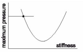
Figure 6. The assumed relationship of the maximum pressure and the material stiffness
