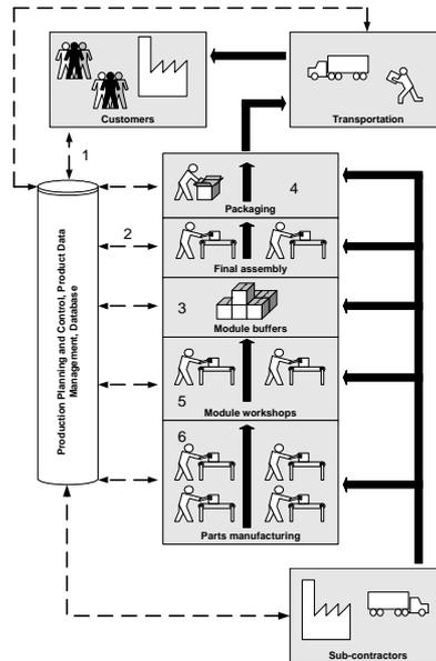
**Figure 1. The Assembly-Initiated Production principle. Solid lines show materials flow, and broken lines show information (Karlsson, 2001)**
