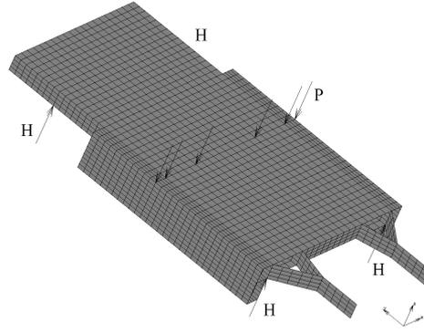
**Figure 2. FE model of the bottom structure of DutchEVO car. P - design load; H – hinges**
