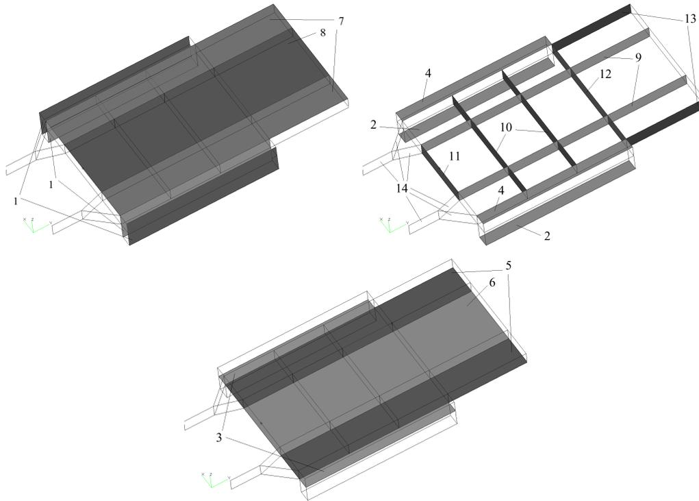
**Figure 1. Structure of the bottom part of DutchEVO car: 1 – vertical and 2, 3, 4 – horizontal components of the side rocker beams; 5, 6 – components of the lower and 7, 8 – upper panels of the floor; 9, 13 – longitudinal and 10, 11, 12 – transverse stiffeners; 14 – backbone profiles**
