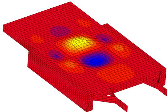
**Figure 4. Buckling of the bottom structure**
