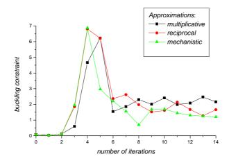
Figure 3. Behaviour of the buckling constraint of different approximation types
