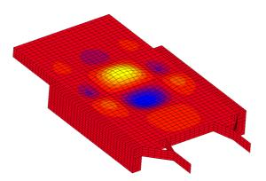
Figure 4. Buckling of the bottom structure
