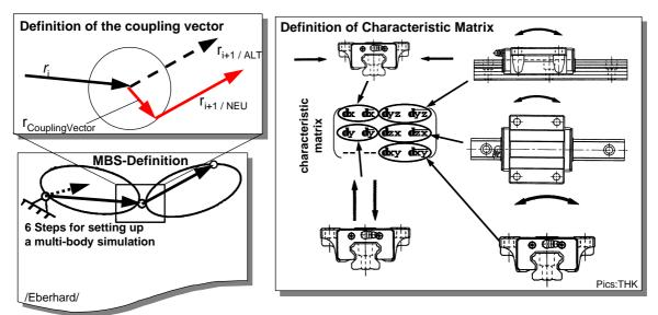
Figure 2. Integration of tolerances, resp. accuracy, into the multi-body simulation
