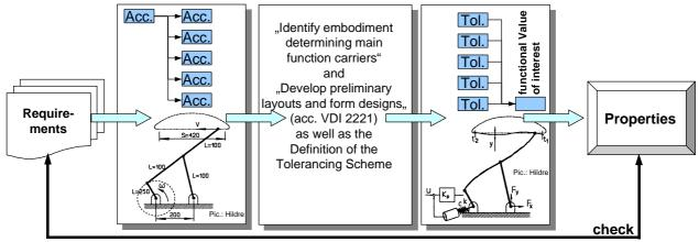
Figure 1. Accuracy and tolerances in the development process
