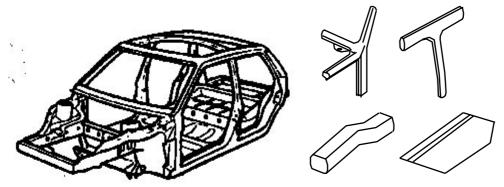
Figure 4. Organ structure of a car uni-body. The car uni-body represents integrated architecture
