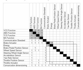
Figure 6. Distributed architecture at organ level, illustrated by automotive active safety systems, ABS, TCS, VSC and BA
