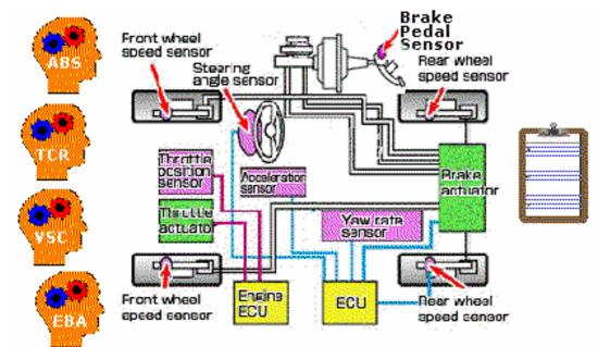
Figure 3. Active safety systems' organs structure. Active safety systems are an example of distributed architecture
