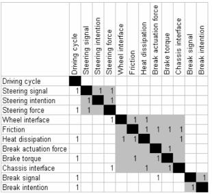
Figure 8. Partially integrated and partially distributed architecture at organ level, applied to chassis systems
