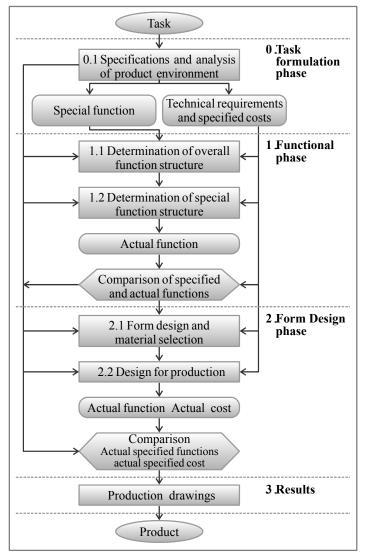
Figure 6. Engineering design process model by Dym
