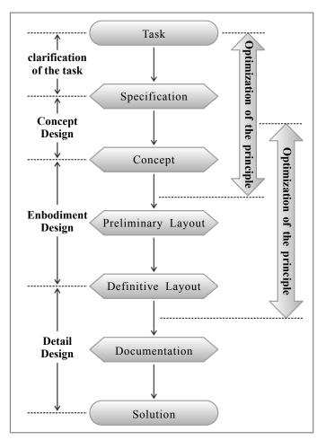
Figure 5. Engineering design process by Phal & Beitz
