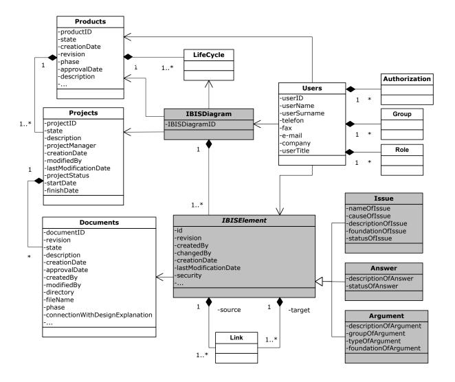
Figure 1. Proposed UML model of IBIS diagrams embedded in PLM system
