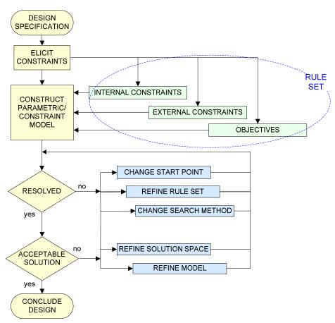
Figure 2. The process of designing with constraints
