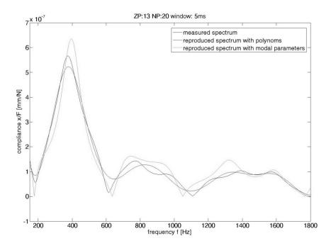
Figure 8. Measured and reproduced transfer function
