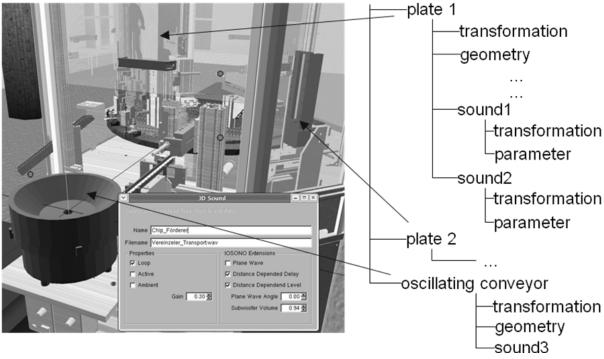
Figure 3. Audio-visual model of a revolving automatic assembly machine
