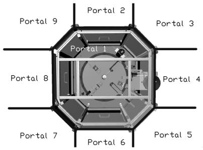
Figure 4. Portals in the model of a revolving automatic assembly machine
