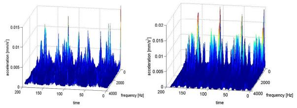
Figure 10. Measured and simulated acceleration on the surface (side wall) of the pick-place unit
