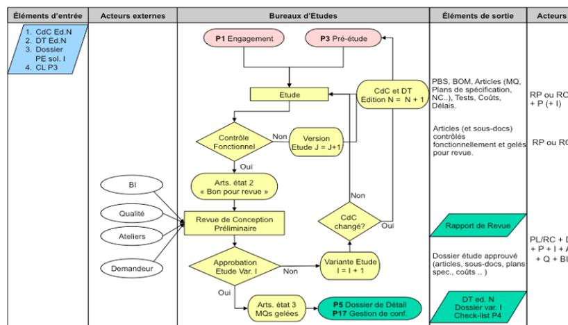
Figure 1. An extract of the mechanical design office process modelling
