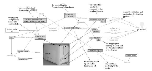
Figure 1. Engineering model of a simple toaster drawn using the new approach in DRed
