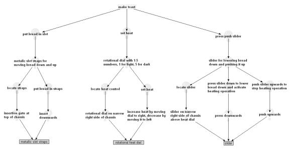
Figure 3. User model of a simple toaster drawn using the new modelling approach in DRed
