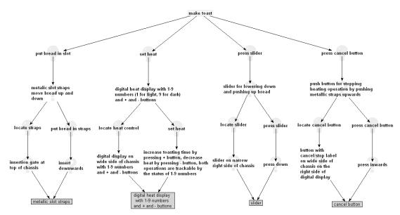
Figure 2. Designer model of a simple toaster drawn using the new modelling approach in DRed
