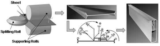
Figure 1. Manufacturing multi-chambered profiles
