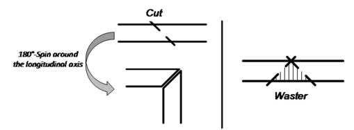
Figure 4. Consequences of symmetric (left) and non-symmetric (right) cross-sections
