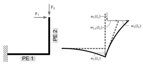
Figure 8. Bending of profile-structures
