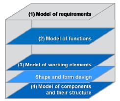
Figure 2. The Munich Model of Product Concretization [Ponn and Lindemann 2008]
