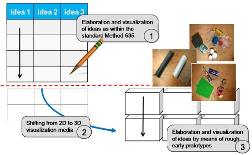
Figure 5. Idea and procedure of adapted Method 635
