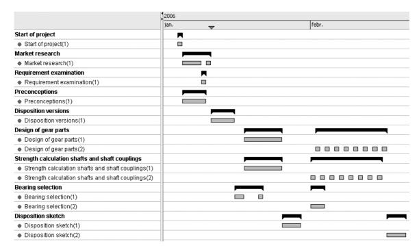
Figure 8: The final Gantt-diagram for the gear drive development process
