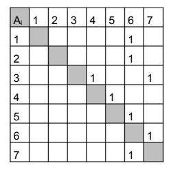
Figure 1: Example of DSM
