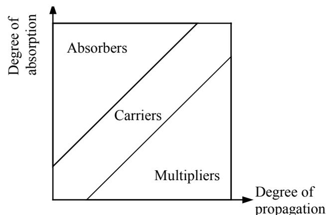
Figure 1. : Change propagation behaviour of parts and systems [ECK-01]
