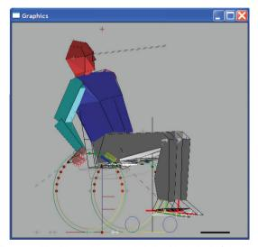
Figure 12 Manikin pushing wheel chair with the ball of the hand
