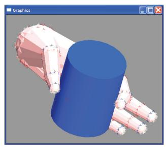
Figure 7 Tip contacts around large cylinder generates cup-like grip.
