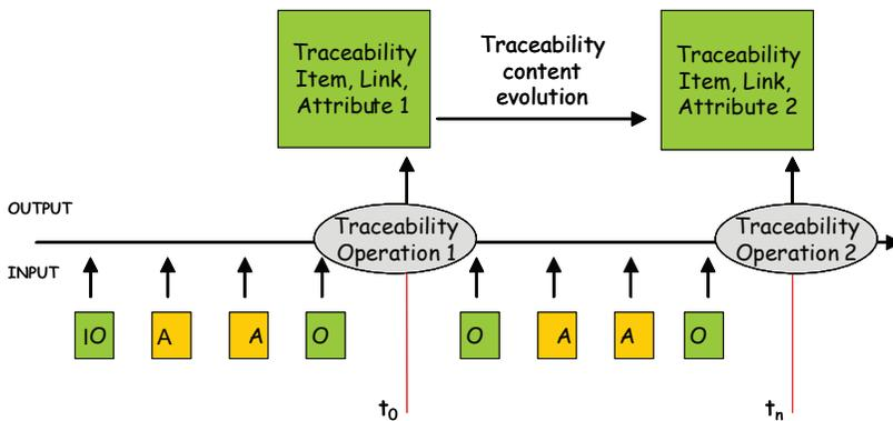
Figure 5. Traceability scenario of development of the information objects in engineering design. The inputs include both information objects and engineering activities.
