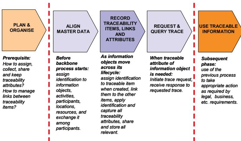
Figure 6. Traceability process in engineering design (after GS1 standard [14])
