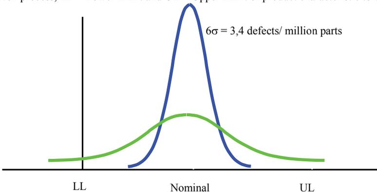
Figure 3 – Process Capability Curve – Conventional versus Six Sigma [8]
