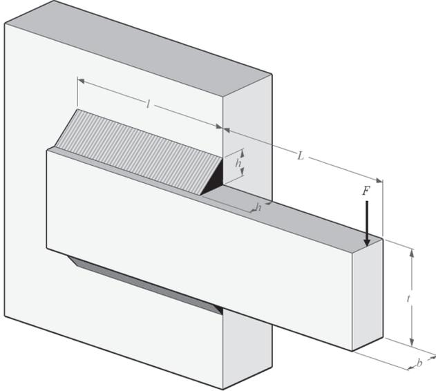
Figure 2. Illustration of the welded beam design
