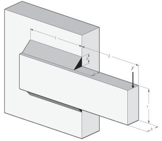
Figure 2.Illustration of the welded beam design
