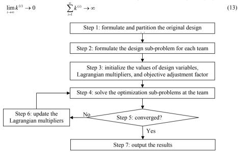
Figure 1. Solution procedure for solving decentralized design problems
