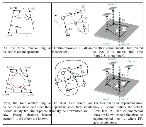
Figure 5: The process of composing a mechanism and its dual pillar system through the duality between the PLGR and FLGR.
