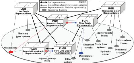
Figure 2: Map of graph representations, their interrelations, and association with engineering systems (Shai and Reich, 2004b). The map includes the relations between mechanisms and determinate trusses that are used in this paper.
