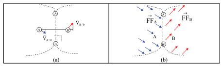
Figure 3: The dualism between joint velocities in a mechanism and the face forces in the dual truss. (a) The primal mechanism and its linear velocities. (b) The corresponding dual truss and its face forces.
