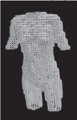
This project has explored the potential to use linked structures to fit around a personalized body shape. Laser Sintering was selected as particularly suitable as it is self supporting during build, because it would have been extremely challenging and time consuming to build a support scaffold for a delicate chain link structure.
