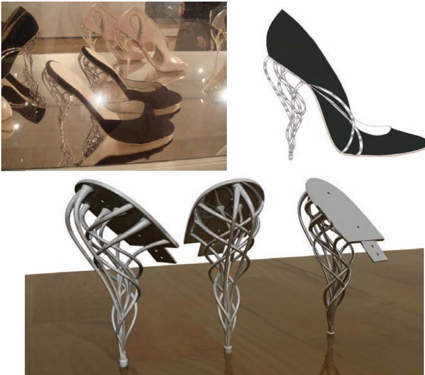
*Figure 2 Rapid prototyping model of the heel, final shoe and sketch above*
