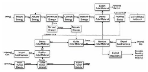
Figure 9. Synthesized conceptual functional model for an automated can opening product
