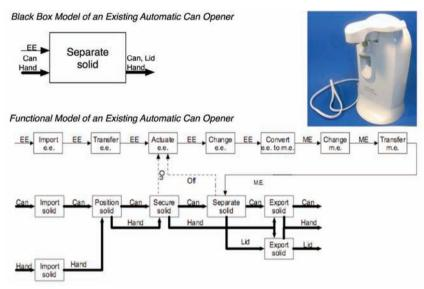
Figure 10. Black box and functional models for an existing automatic can opener<sup>2</sup>
