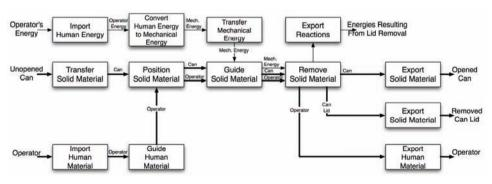
Figure 3. Functional model of a manual can opener
