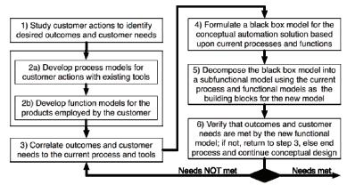
Figure 7. Approach for the development of conceptual functional models for automating processes
