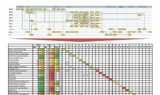
Figure 6. Process map and evaluated dependency matrix of a real-life example
