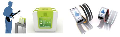
Figure 2 'Musicube', is a device that teaches people how to play guitar in a playful way. The wireless glove provides visual and tactile feed back (Fröbelspaces). The "PartyBracelet" is used in discos to support the communication between members of related groups and the interaction with lighting and music (Tribeware).
