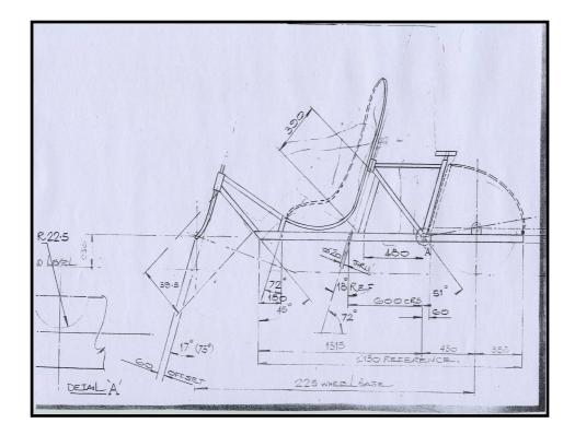
Figure 1 Layout of Tandem with Main Dimensions
