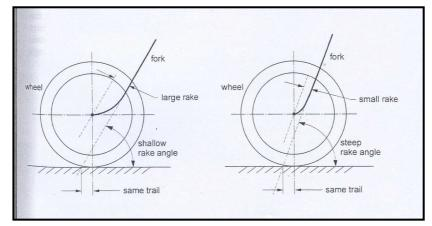
Figure 2 Steering Geometry
