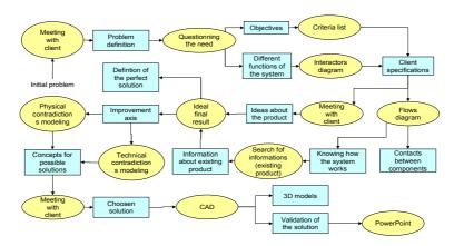
Figure 1: Example of effective paths between tools (ellipses) and results (rectangles)
