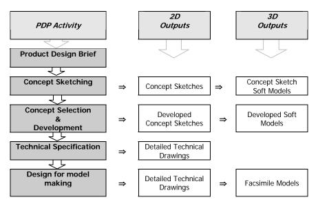
Figure 1: A simplified version of the "traditional" UWIC PDP showing typical 2D & 3D design outputs for each activity
