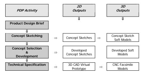
Figure 2: A simplified version of the "computerised" UWIC PDP showing typical design outputs for each activity
