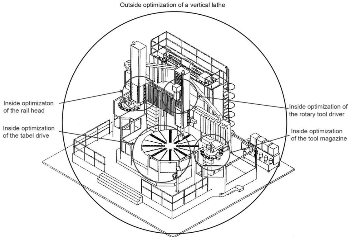
**Fig. 3 Outside and inside optimization of a vertical lathe made by TOSHULIN company**
