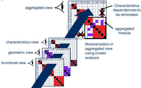
Figure 3. 3D-Clustering of component dependencies, derived from Multiple-Domain Matrix
