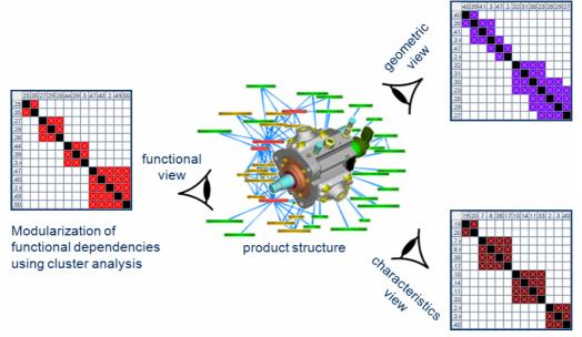
Figure 2. Different views on the product structure derived from a Multiple-Domain Matrix
