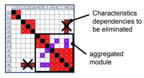
Modularization in aggregated view using cluster analysis
