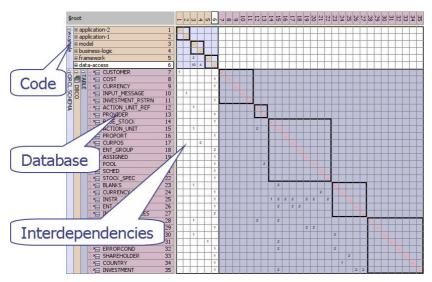
Figure 1. Multi-domain DSM of Application with Database
