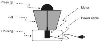
Figure 1: Conceptual representation of an electric fruit juicer
