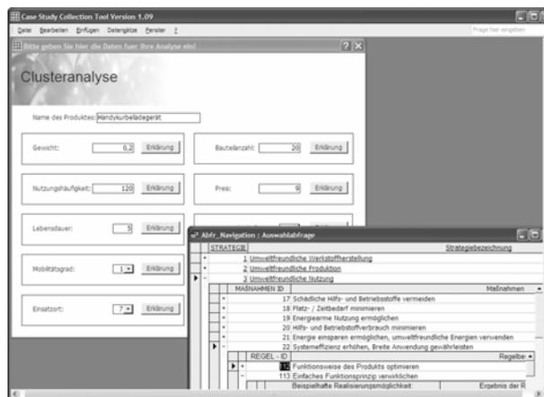
Figure 3: *Case Study Collection*. The upper left window in the background shows the input mask for entering functional parameters, the window to the lower right in the foreground permits to navigate through the design strategies, design measures and design guidelines.
