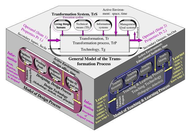
Figure 3 Transformation Models – a general principle adapted to the design process and teaching & learning process
