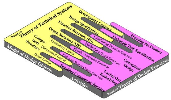
Figure 6 Design Object Model and Design Process Model – Comb Model
