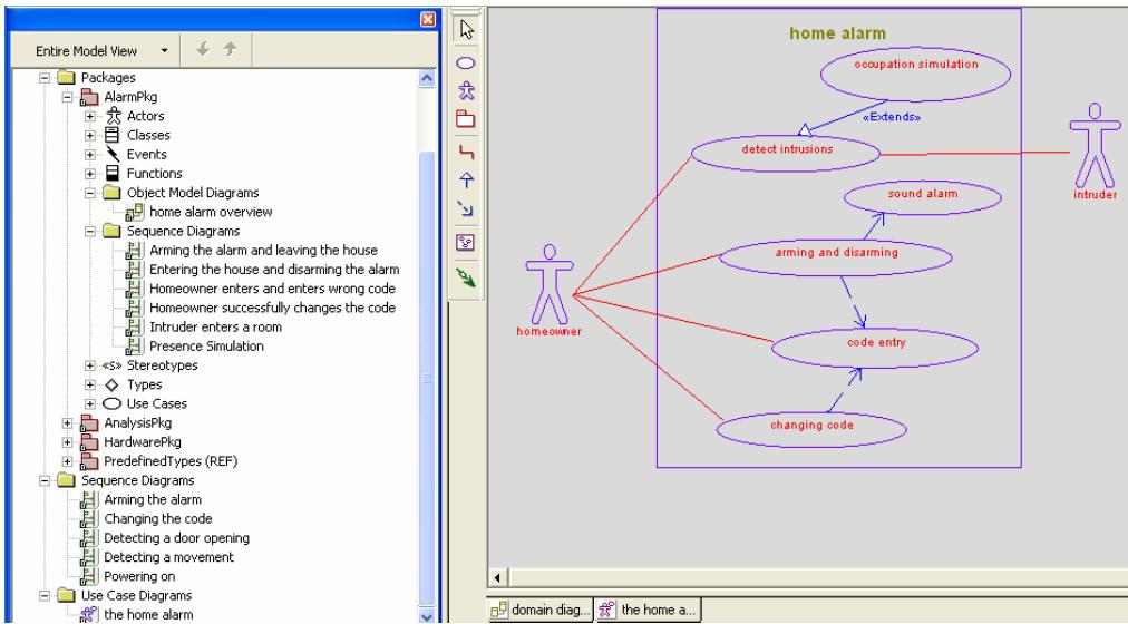
Figure 1. Example of a SysML model and a use case (Home Alarm)
