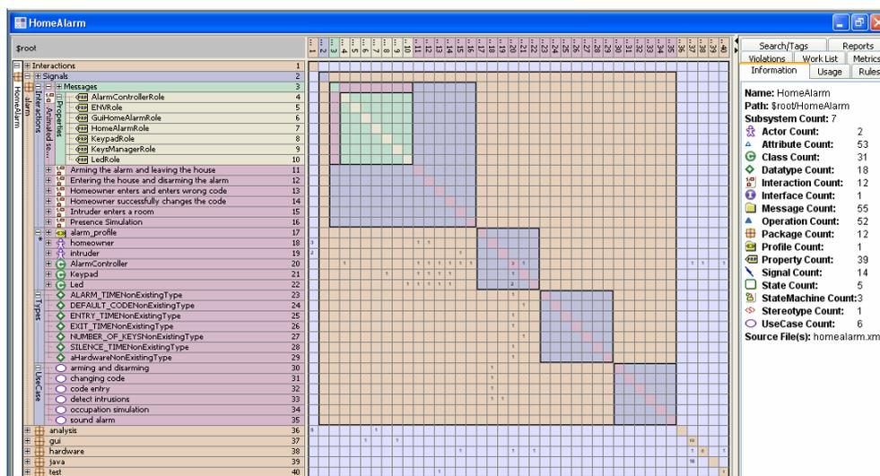
Figure 2. DSM of the Home Alarm SysML model
