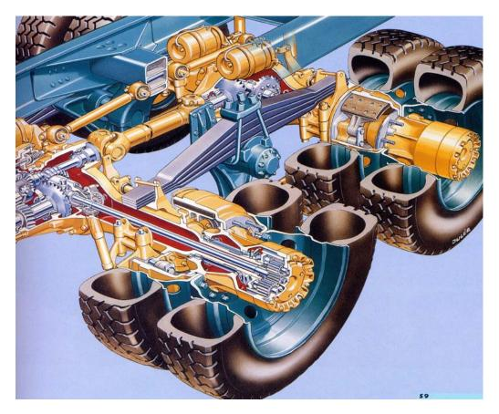
Figure 4 Illustration of the rear of a Scania truck
