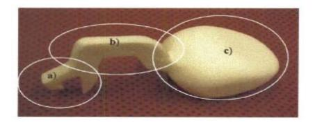
Figure 1. Model showing three functional surfaces of a bottle opener: a) a technical functional surface, b) a communicative constrained functional surface, and c) an ergonomic functional surface. Photo: C.M Johannesson.
