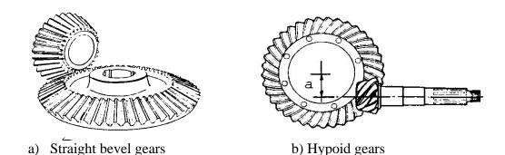
Figure 7. Bevel gears
