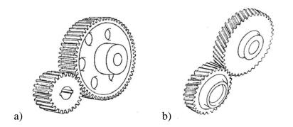
Figure 6. Cylindrical gears with parallel shafts: a) Spur gears, b) Helical gears
